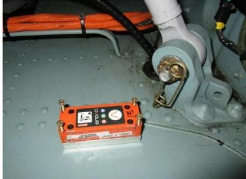
Each Slamstick S4-E100D40 sensor holds three piezoelectric accelerometers (+/- 100 g), and was configured with a sampling frequency of 8192 Hz.
