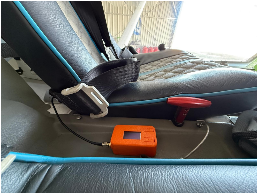
ADS-L HDR-only transmitter installed in the cockpit, the coax leads to the external antenna at the bottom of the aircraft
