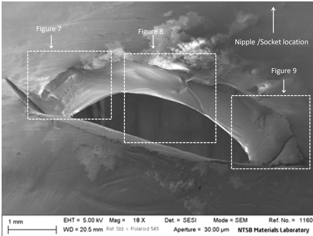
Figure 5. SEM image of crack with areas of interest highlighted.
