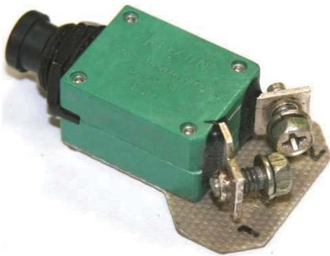
**Figure 6:** BACC18AZ7R circuit breaker in the “as received” condition.
