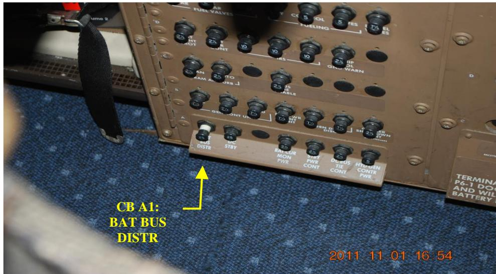
Figure 25. P6-1 panel in the cockpit (section with C829 circuit breaker).
