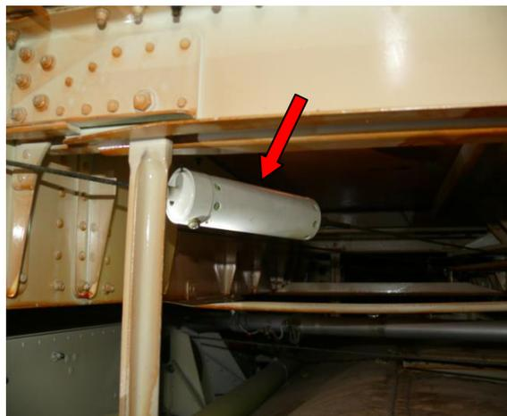
Figure 21. Load limiter of the alternate landing gear extension system (right main gear).
