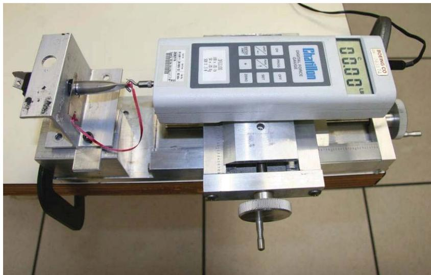
Figure 12: Operating force test setup.
