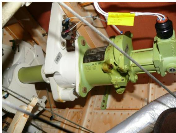
Figure 18. Electric actuator of the alternate landing gear extension system (Source - SCAAI).
