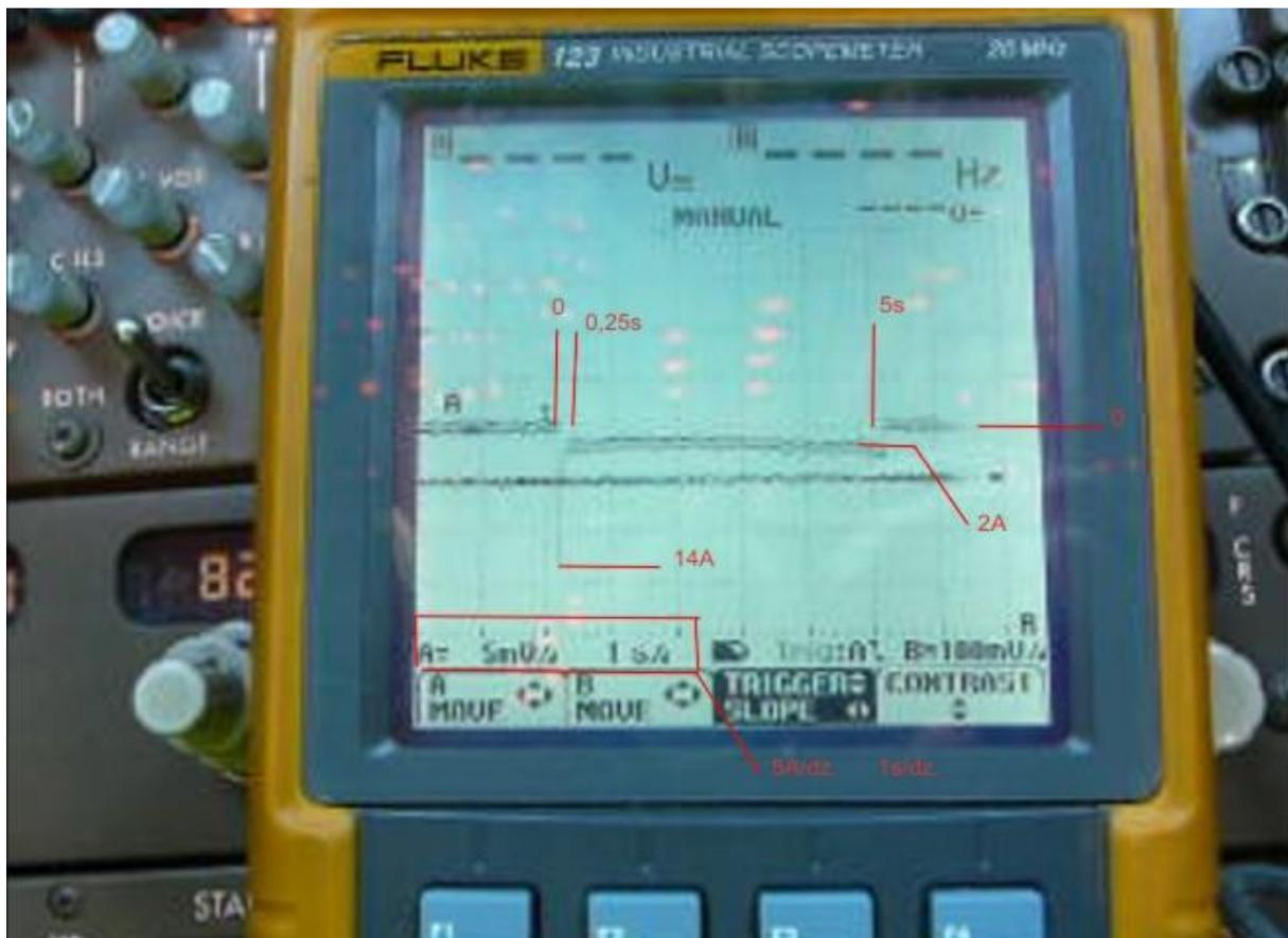
Fig. 5. Recorded waveform of the current of the alternate landing gear extension motor
