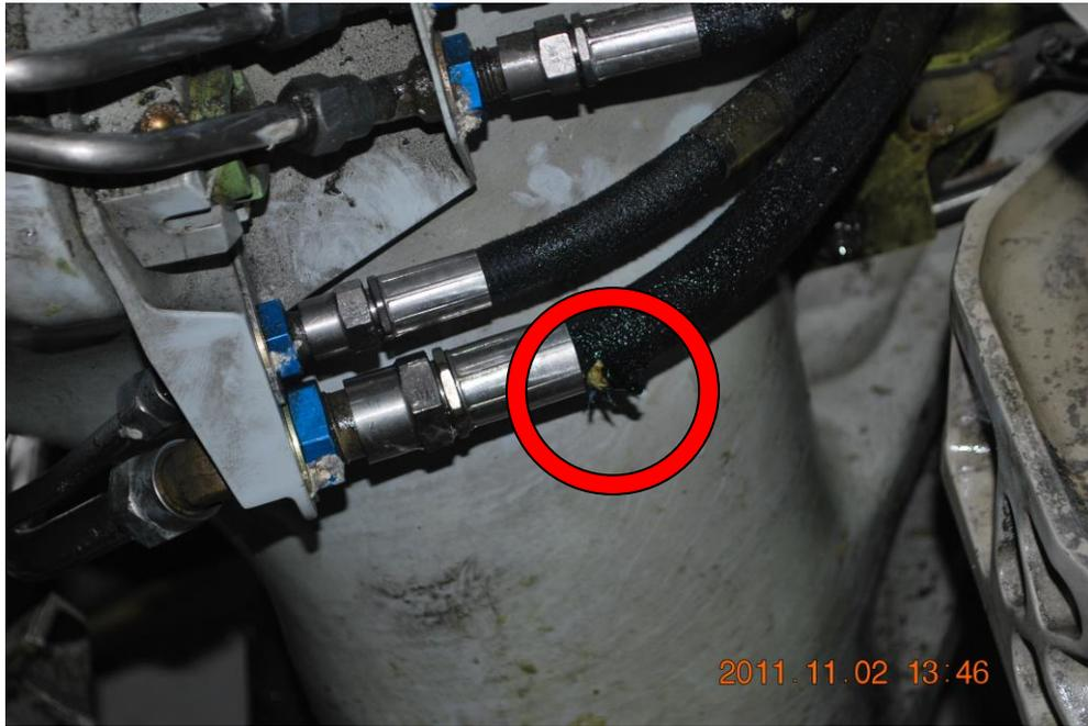
Figure 23. Close-up of the damage to the hydraulic hose (marked with red circle) on SP-LPC right main gear. (Source – SCAAI)
