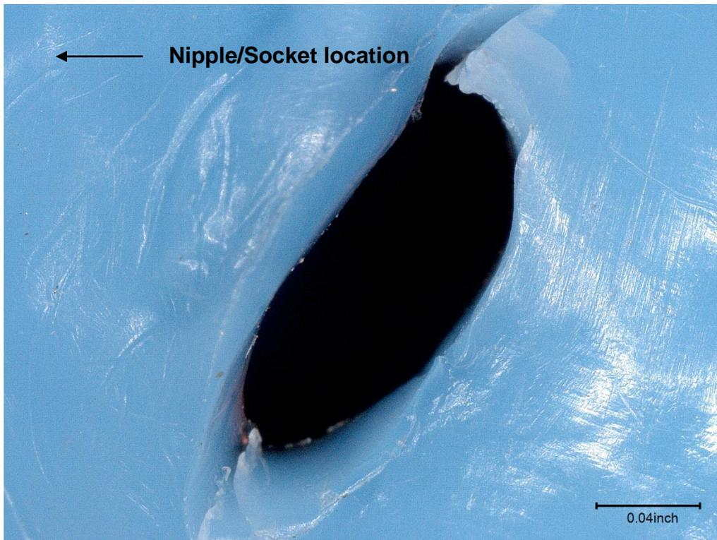
**Figure 4. Close-up photograph of crack in hose sidewall.**
