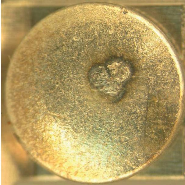
**Figure 25:** BACC18Z7R moveable contact 1.
