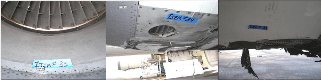
Figure 3. Damage to the left engine nacelle – from the left: fan inlet inside, bottom part, thrust reverser.
