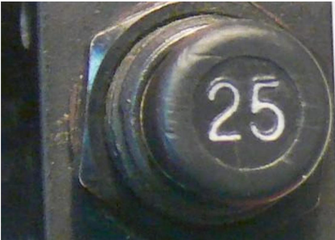
Fig. 10. Button of C829 circuit breaker from SP-LPC airplane
