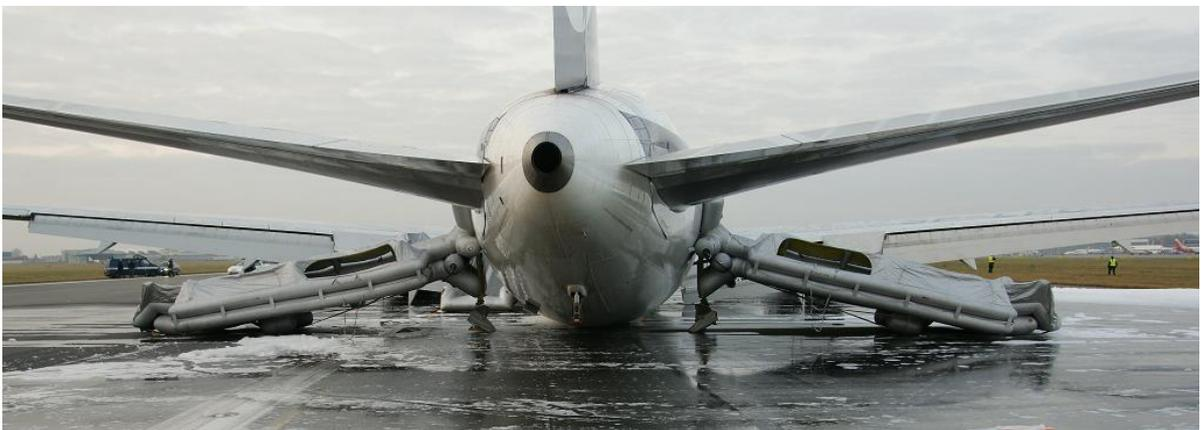
Figure 16. Setting of the rear slides of SP-LPC airplane after emergency landing.
