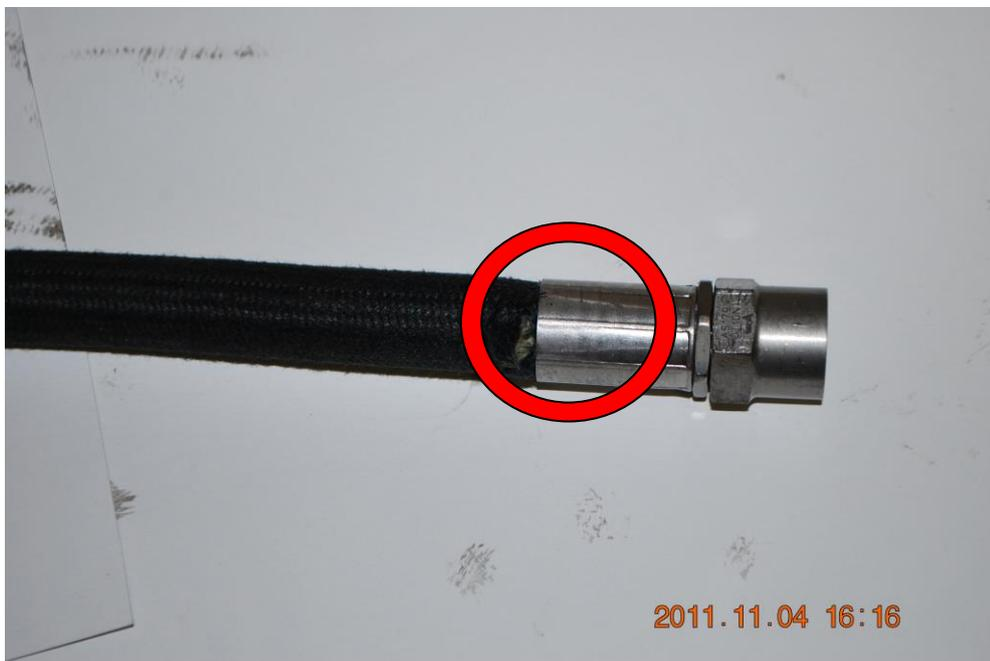
Figure 24. Damage to the hose from hydraulic system of SP-LPC airplane. (Source – SCAAI)
