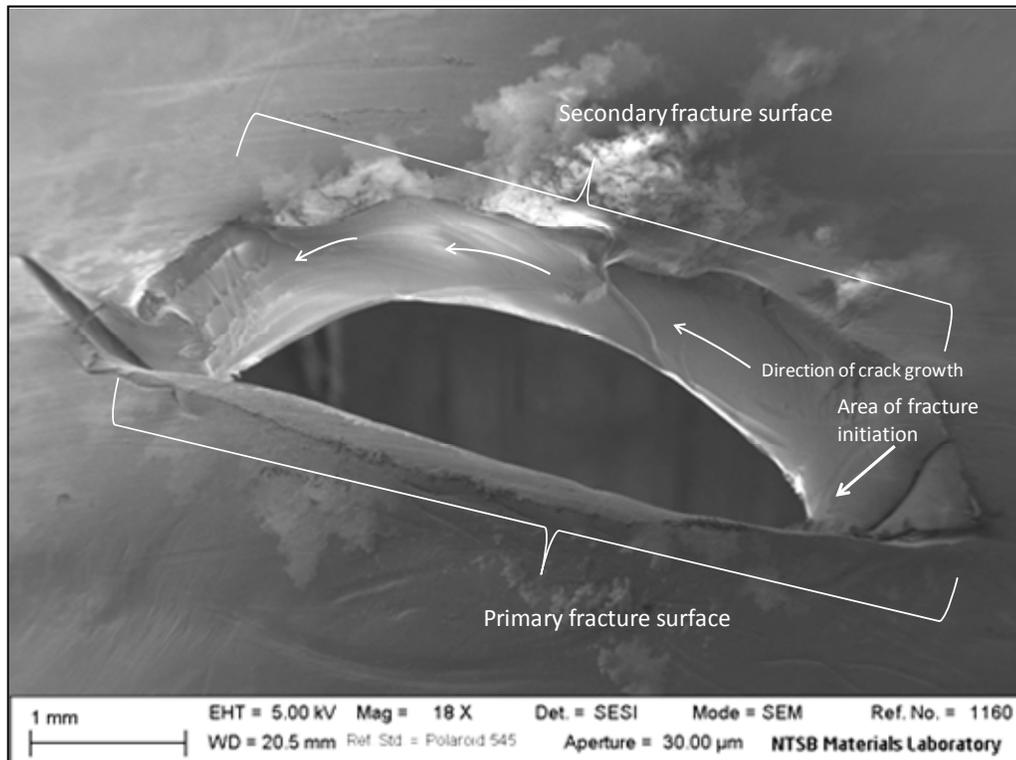
Figure 6. SEM image of crack with fracture features annotated.
