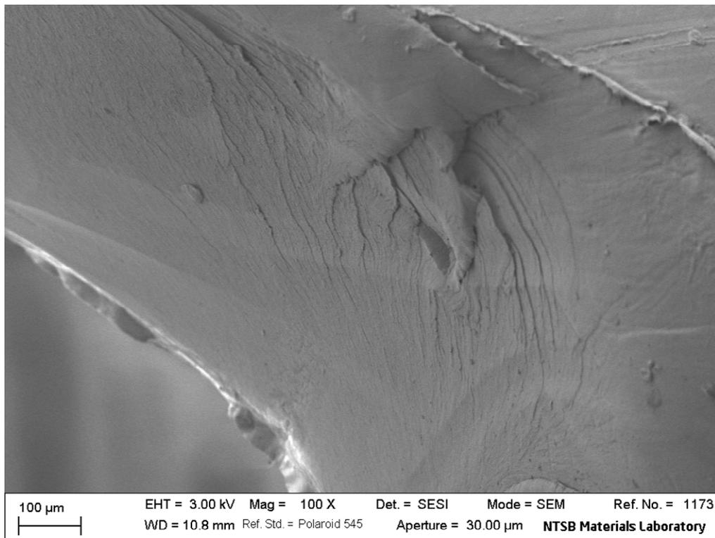
**Figure 10. Close-up SEM image of branch cracking and directional crack markings.**
