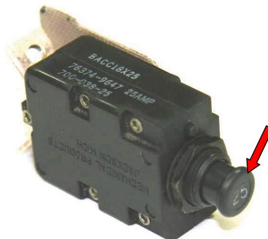
Figure 5. C829 circuit breaker removed from SP-LPC airplane. The circuit breaker in the ON/pressed setting. Red arrow indicates the circuit breaker head (Source –Boeing).
