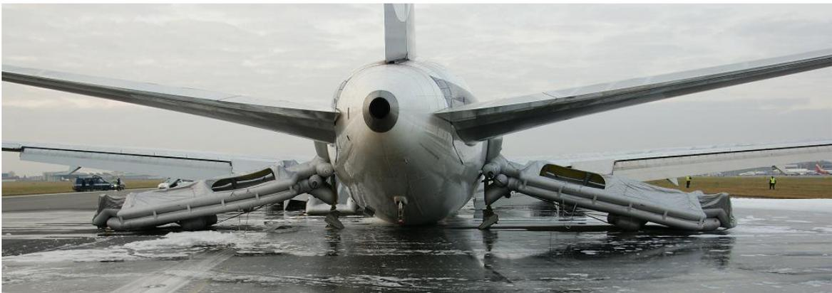
Figure 4. Position of the aft slides of SP-LPC airplane after gear up landing.
