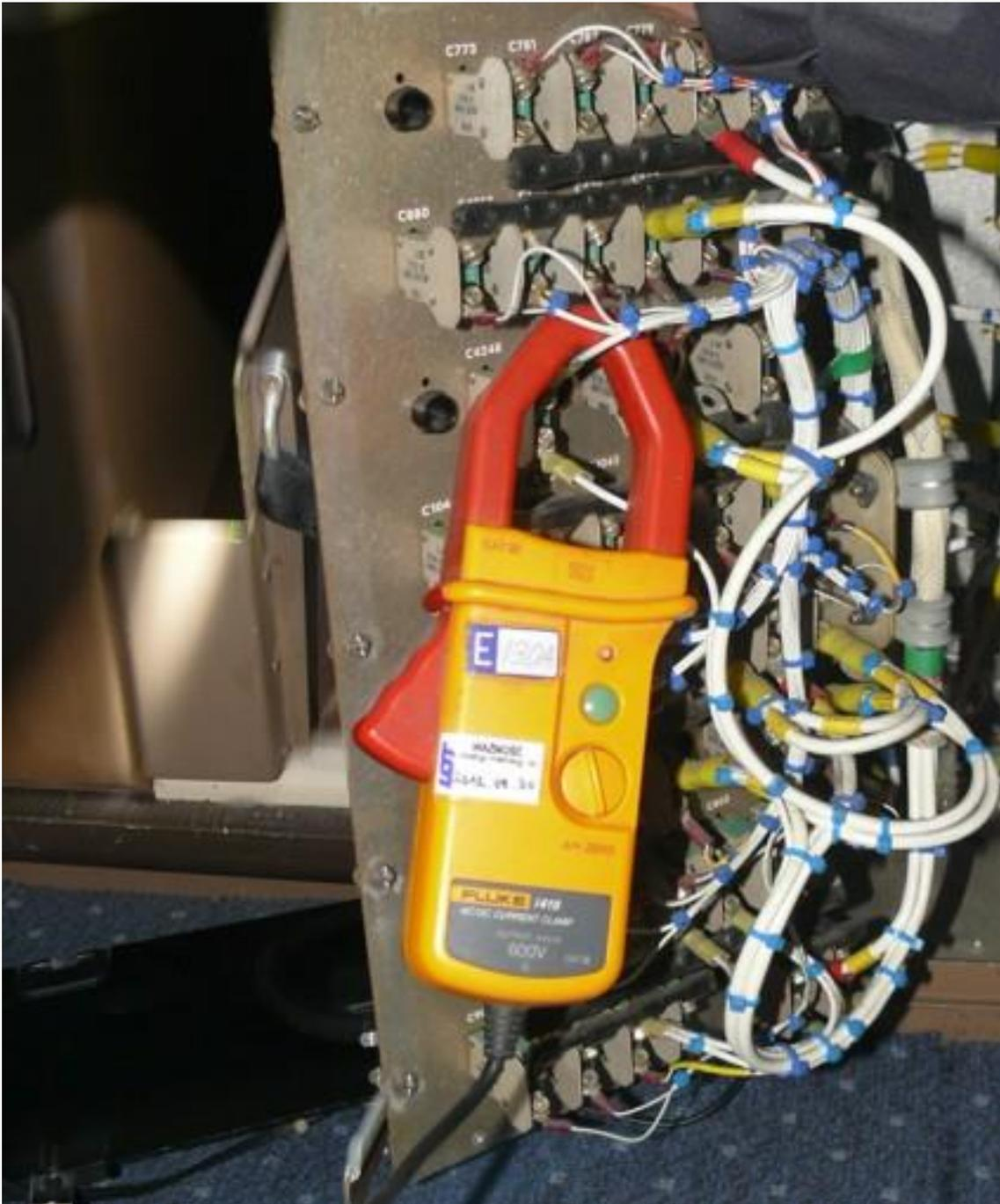
Fig. 6. Connecting of a clamp ammeter probe to the circuit of the C4248 circuit breaker
