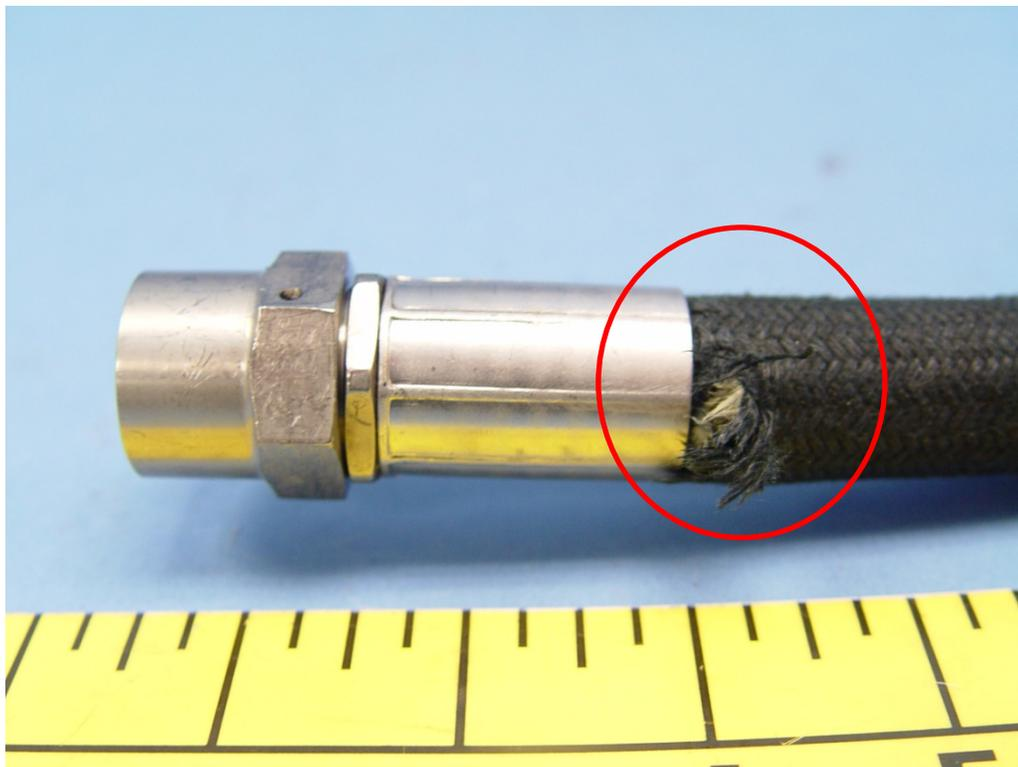
**Figure 2. Close-up photograph of damage to hydraulic hose (area highlighted in red circle).**
