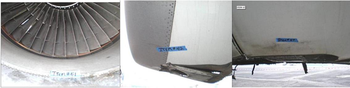
Figure 4. Damage to the right engine nacelle – from the left: fan inlet inside, bottom part, thrust reverser.
