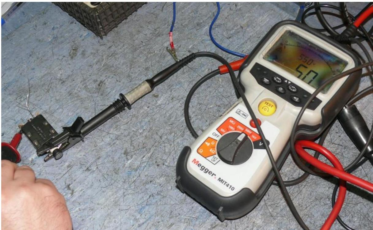
Fig. 12. Measurement of insulation resistance of C829 circuit breaker
