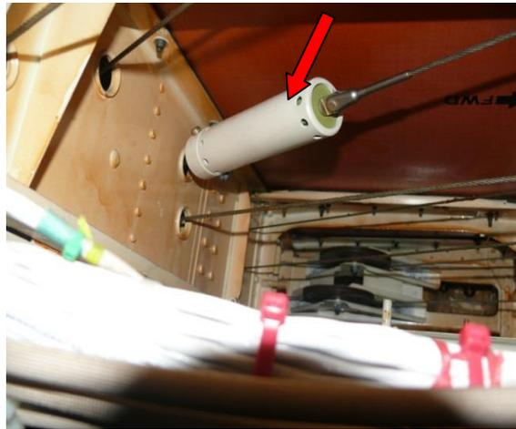
Figure 20. Load limiter of the alternate landing gear extension system (left main gear).
