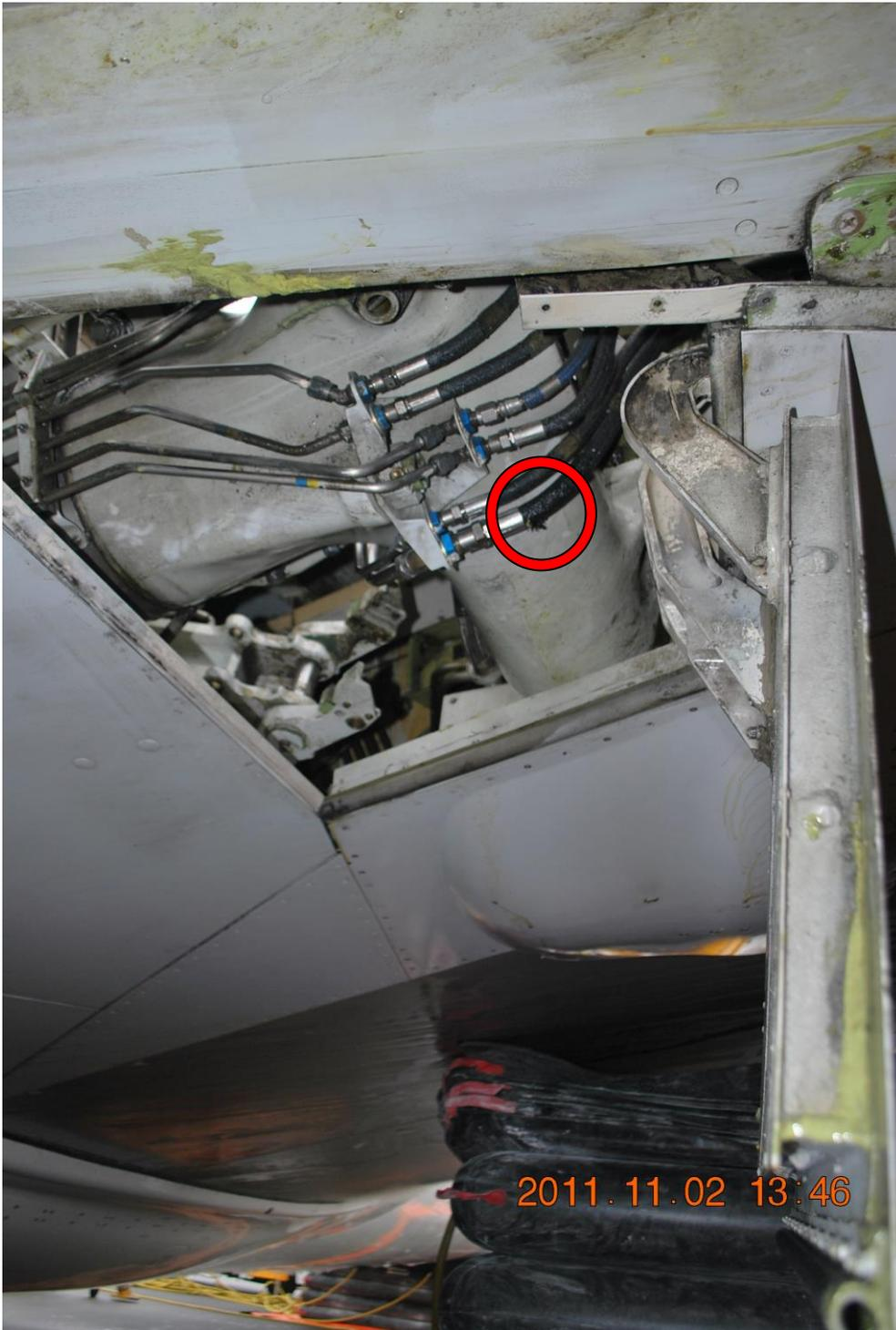
Figure 22. Damaged hydraulic hose (marked with red circle) on SP-LPC right main gear.
