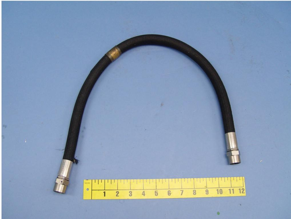
**Figure 1. Overall photograph of accident hydraulic hose.**
