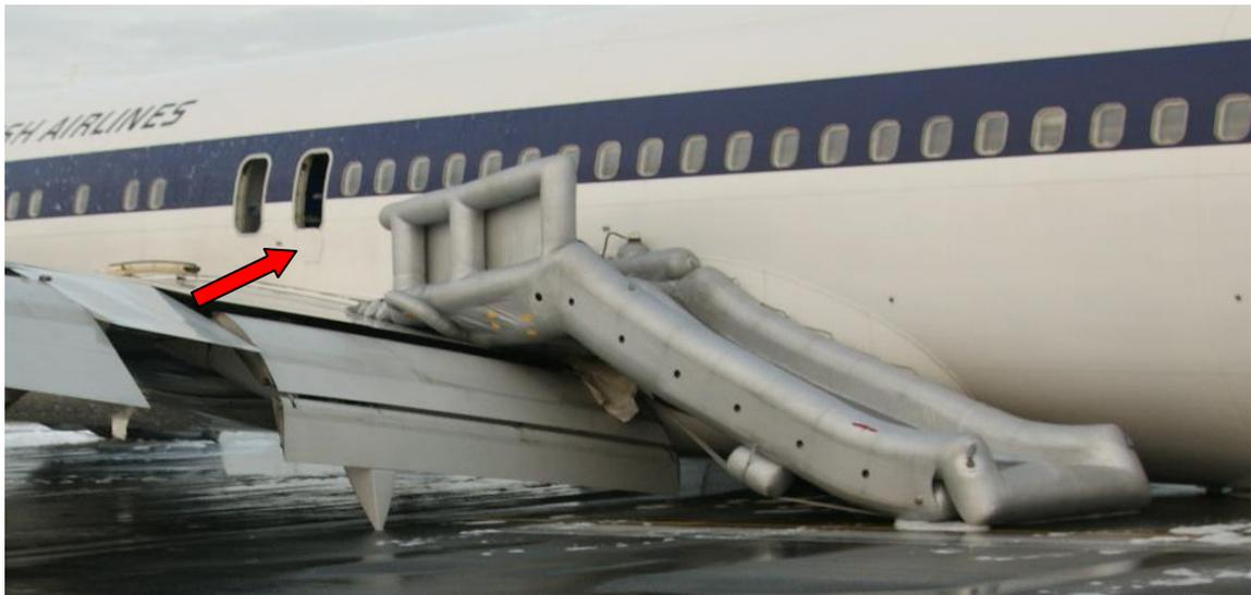
Figure 5. Evacuation slide on the left wing and locked drop step.
