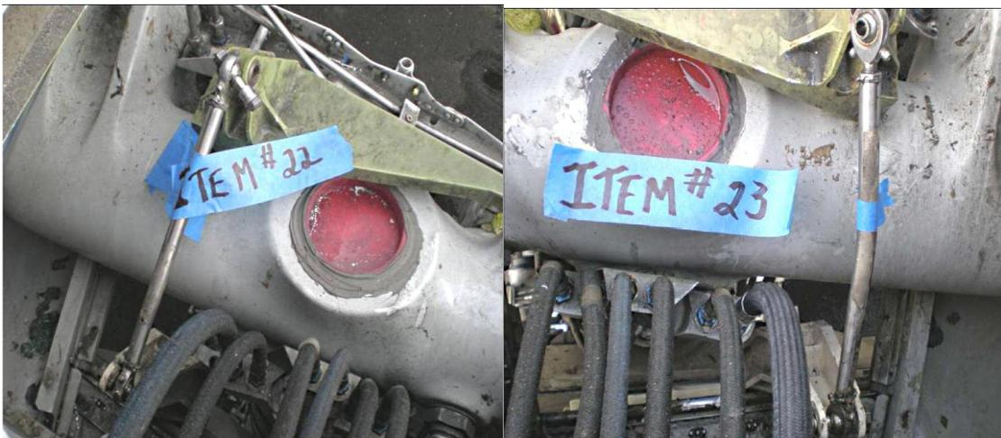
Figure 2. Damaged struts of the main landing gear hatch door (left and right).
