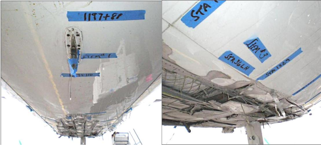
Figure 1. Damage to the lower part of the fuselage in the area of section 46 – front view and close up.
