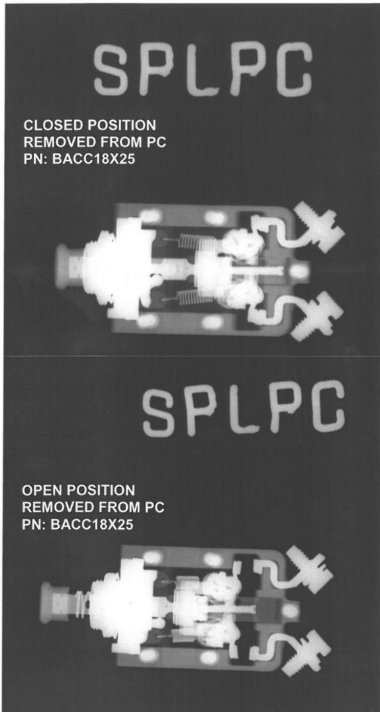
Fig. 8. X-ray picture of C829 circuit breaker
