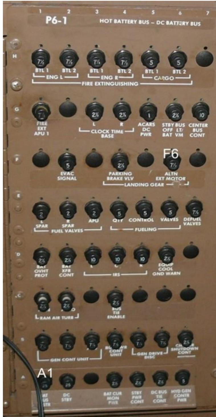
Figure 6. P6-1 panel. A1 - C829 BAT BUS DISTR circuit breaker and F6 – C4248 LANDING GEAR – ALTN EXT MOTOR
