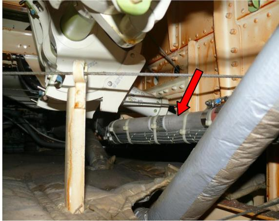
Figure 19. Load limiter of the alternate landing gear extension system (nose gear).
