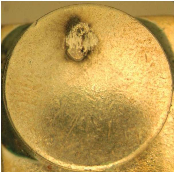
**Figure 23:** BACC18Z7R fixed contact 1.
