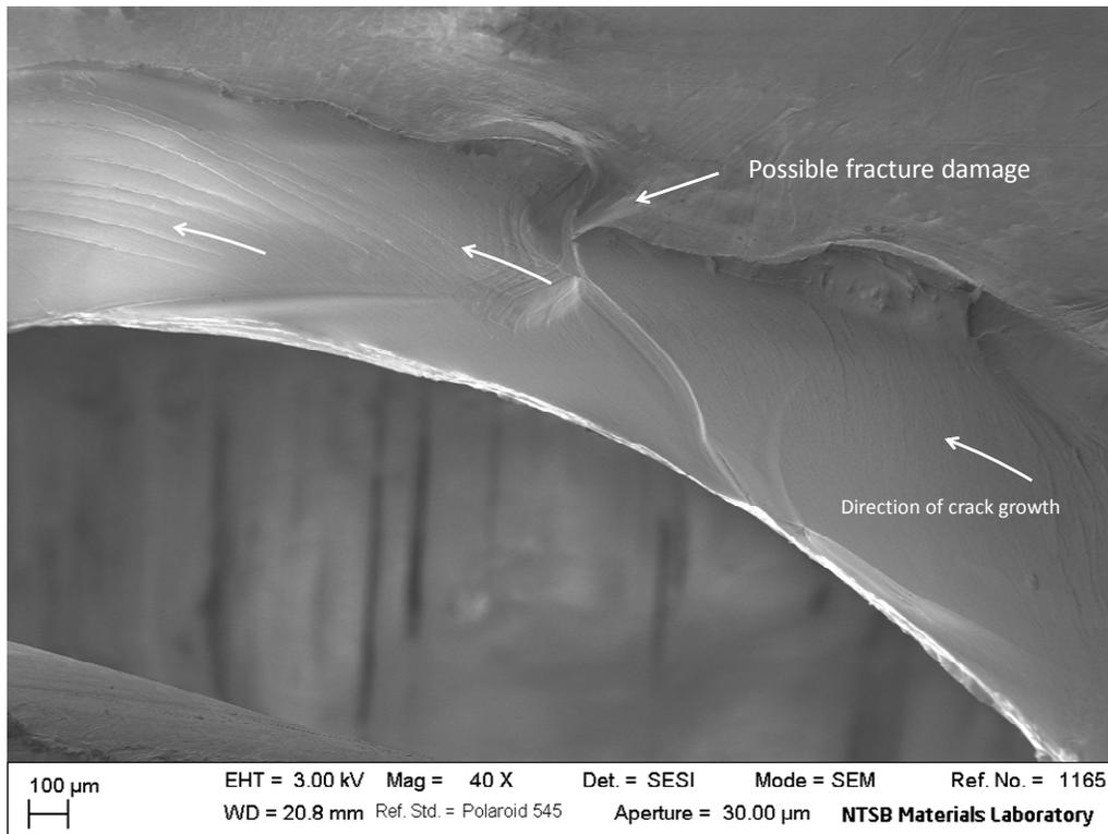
Figure 8. SEM image of center section of secondary fracture surface.
