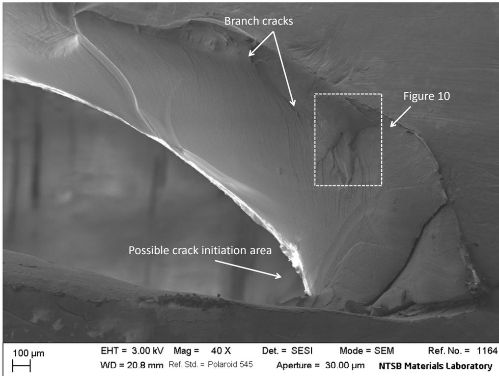
**Figure 9. SEM image of center section of secondary fracture surface and crack initiation area.**
