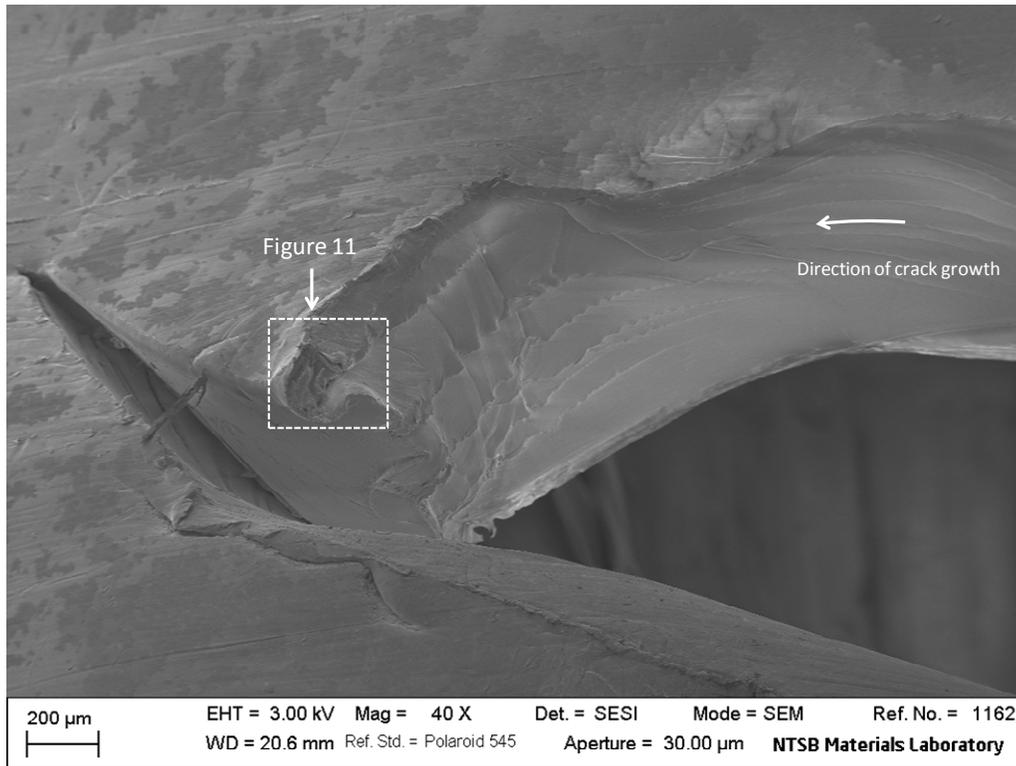
Figure 7. SEM image of left side of secondary fracture surface.
