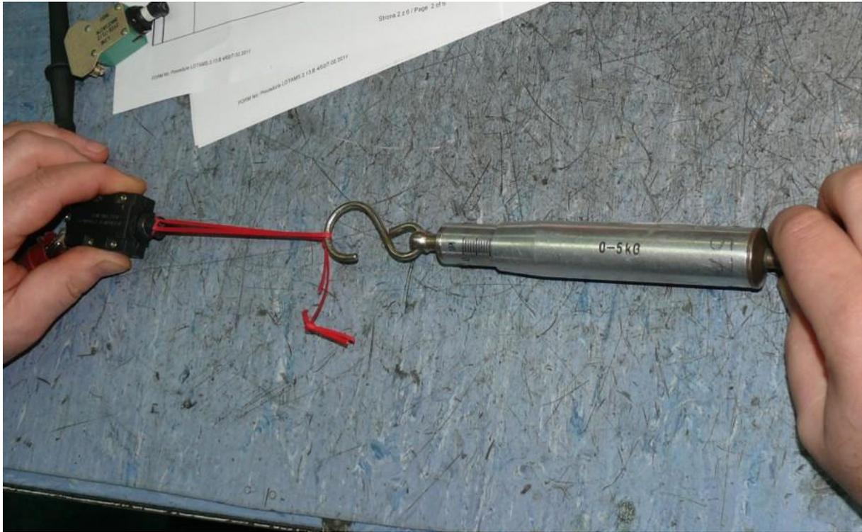
Fig. 11. Measurement of pull-out force (OFF setting force) of C829 circuit breaker
