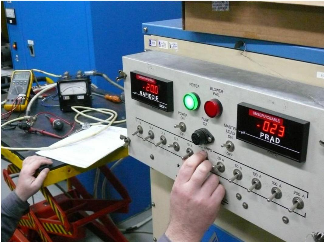
Fig. 13. Measurements of currents of C829 circuit breaker
