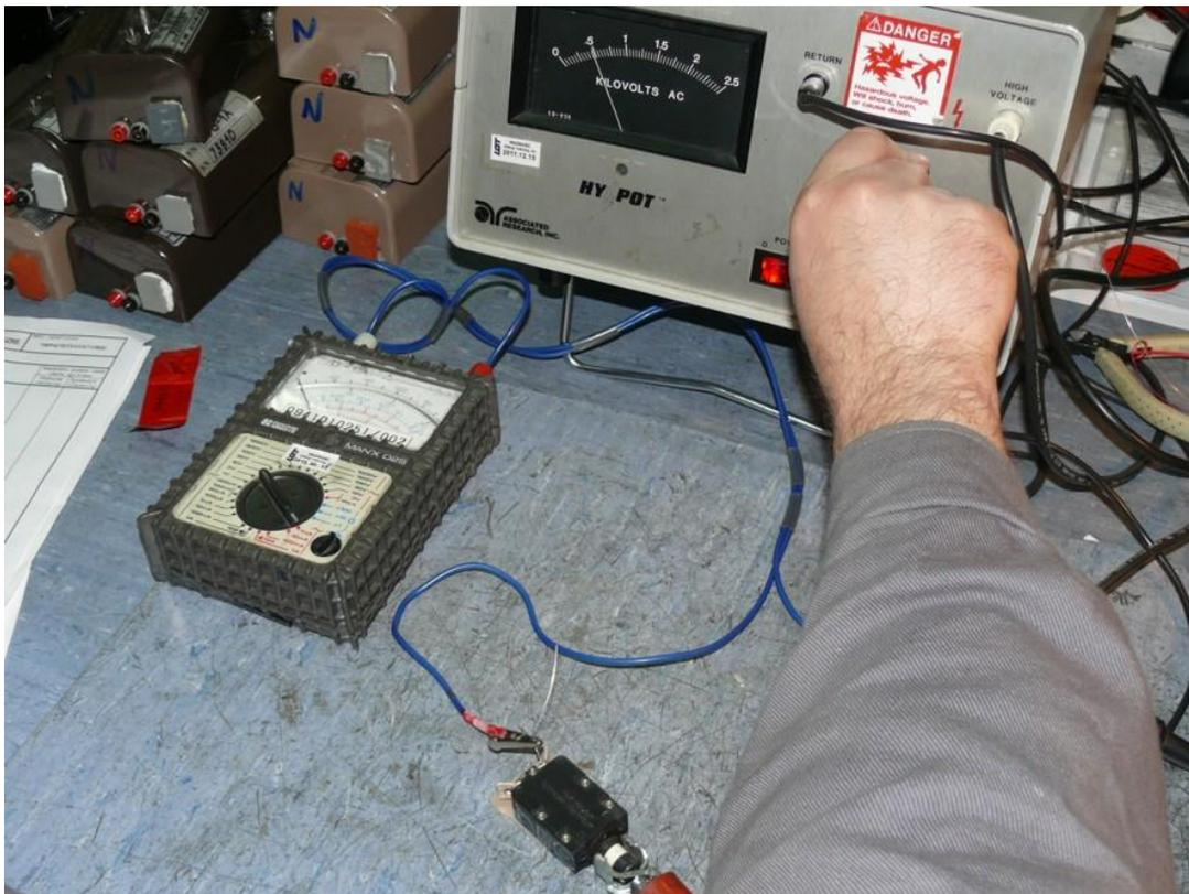
Fig. 14. Measurement of dielectric leakage current of C829 circuit breaker
