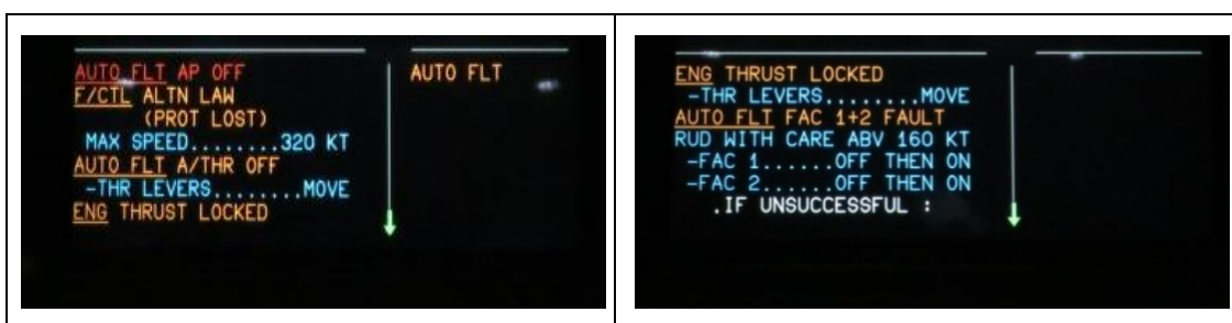
Figure 33: The page 1 and 2 of the ECAM messages after CBs of FAC 1 and 2 being reset
