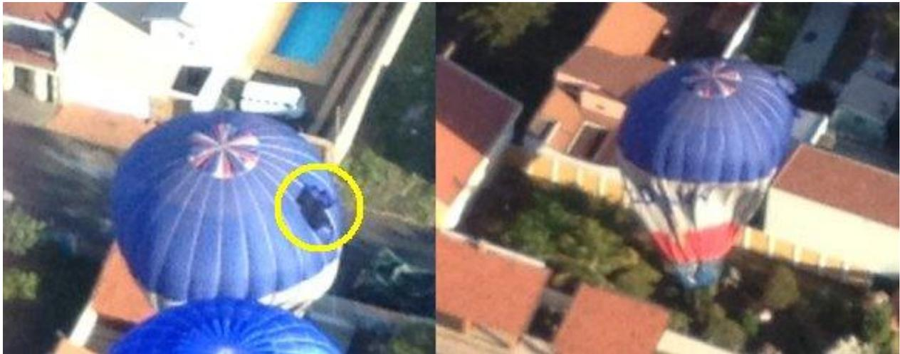
*The left photo shows the damage to the upper part of the SP-BBP envelope. The right photo shows SP-BBP landing with the envelope only partially inflated.*
